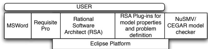
Figure 1. The EuRailCheck architecture.
