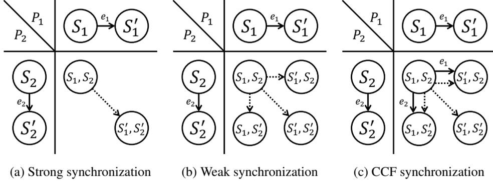
Figure 3: AltaRica synchronizations: in each figure the bottom right corner represents the allowed transitions in the composition of the two systems. Dashed arrows represent a transition where both  $P_1$  and  $P_2$  move (i.e. the fired event in the composition is  $e_1/e_2$ ), while solid arrows represent a local transition.
